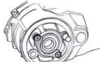
Remove oil seal with the special tools.
