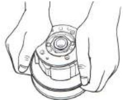
*Warning:* Gradually back off the clutch shoe assembly pressed down by hands to reduce the clutch-spring load.
