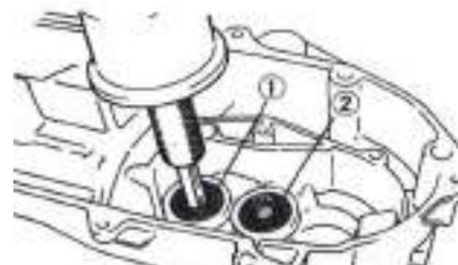
*Caution:* The removed bearings should be replaced with new ones.
