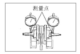
Check if the crank shaft is noisy or loose while restori Replace it if so.
