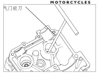
Clear carbon accumulated within the combustion chamber and valve, and thoroughly clean the intake and discharge valves.
