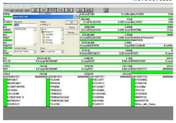
(4) Select "Parameter File" under "Setup", then click "MT05common.par", and then select "Comm protocol" under "Setup", select "Keyword2000" and click "Ok", and select 17 under Device Code at the same time.
