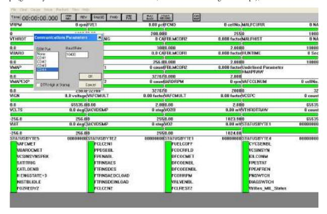
Then the software interface will recover communication, display current fault code at "MALFCURR" and past fault code at "MALFHIST", and inquire the corresponding faults as per the List of Fault Codes.
