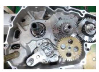
Remove the auxiliary shaft nut, sprocket and sleeve.
