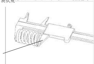
Measure the outer diameter of valve rod. Allowable limit: air inlet: Φ4.955 mm
