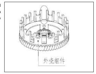
Check whether it is damaged in the dents of the pressure plate and the center bearing support. Replace it if it is damaged.
