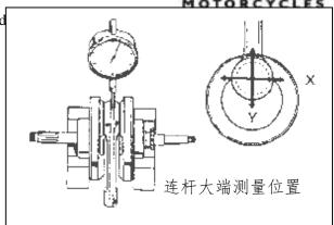
Measure the dislocation of the crank shaft. Allowable limit: 0.03mm
