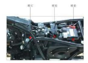
Remove the fixed screw on the air cleaner cover
