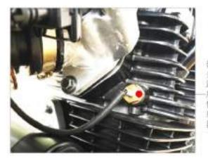
14.2.4.1 Appearance of temperature sensor at cylinder end
