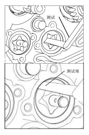
Check rotor end surface stroke Allowable limit: 0.15 mm
