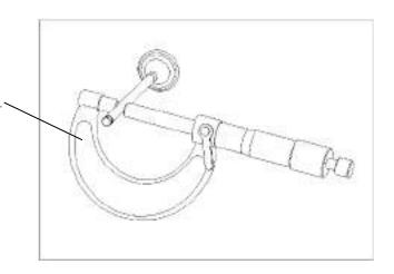
Check the valve guide. Prior to check, use a reamer to eliminate carbon accumulated within the guide.
