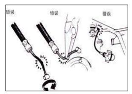
Plastic parts may deteriorate due to aging, which are apt to be damaged by solvent or oil. Check before re-installation and replace if necessary.
