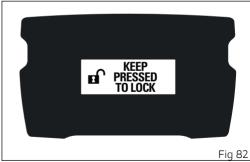
After this 3 second time, if steering lock is properly engaged, the message "STEERING LOCKED" will be displayed on instrument panel.
