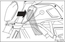
Unscrew the filler plug (2) of the expansion reservoir, on the motorcycle's right side, and add ENI Agip Permanent Spezial antifreeze (do not dilute, use pure), until reaching the MAX level. Screw plug (2).
