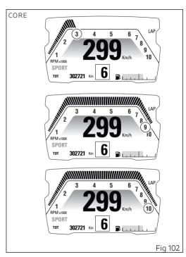
CORE layout indicates rpm in a different way compared to TRACK and FULL layouts.
