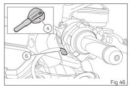
Key-On/Key-Off using the button on the Hands free lock with the passive key
