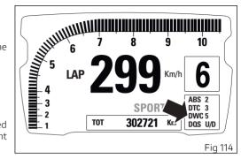
reaction to wheelies. Each Riding Mode features a pre-set intervention level. Level eight indicates a setting that minimises motorcycle tendency to shift up in a wheelie and maximises reaction to the same, if it occurs. While level one is for expert riders and features a lower wheelie control in terms of prevention and less strong reaction to the same, if it occurs.
