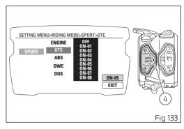
When entering the function, the currently set DTC level or status is indicated on the right (above the word EXIT) (e.g.: ON - 05, i.e. level 05). Customisation options are indicated on the central drop-down menu: levels 1 to 8 and status OFF.
