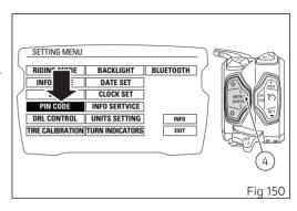
When entering the function, the display shows the message INSERT NEW PIN CODE followed by the first digit in green and three dashes "0 - - - ".
