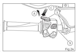
High/low beam switching off during vehicle start (version without DRL light).
