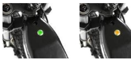
65% and red when the battery charge reaches 30%. The red light will start blinking when the battery charge is very low. From this point, the bike will start losing power and will be able to travel roughly 2 - 3 km (1 - 2 miles) before the motorcycle shuts down completely.
