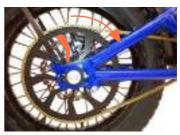
Using the Allen wrench #4 (or Torx wrench #30) loosen and remove 3 bolts holding the motor in the frame.
