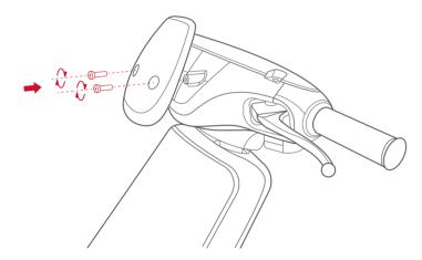
Install the rearview mirrors into the mounting holes on dashboard and turn it clockwise. The bolt shall be screwed in for more than 15mm.
