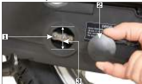
(1) Drive chain (2) Hole cap (3) Drive chain slack 25 mm
