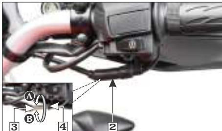
(2) Boot (3) Adjuster (4) Lock nut (A) Decrease free play (B) Increase free play
