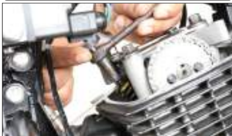
(5) Feeler gauge (6) Adjusting screw (7) Valve stem (8) Lock nut
