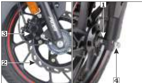
(1) Side collar (2) Disc (3) Caliper (4) Front axle nut
